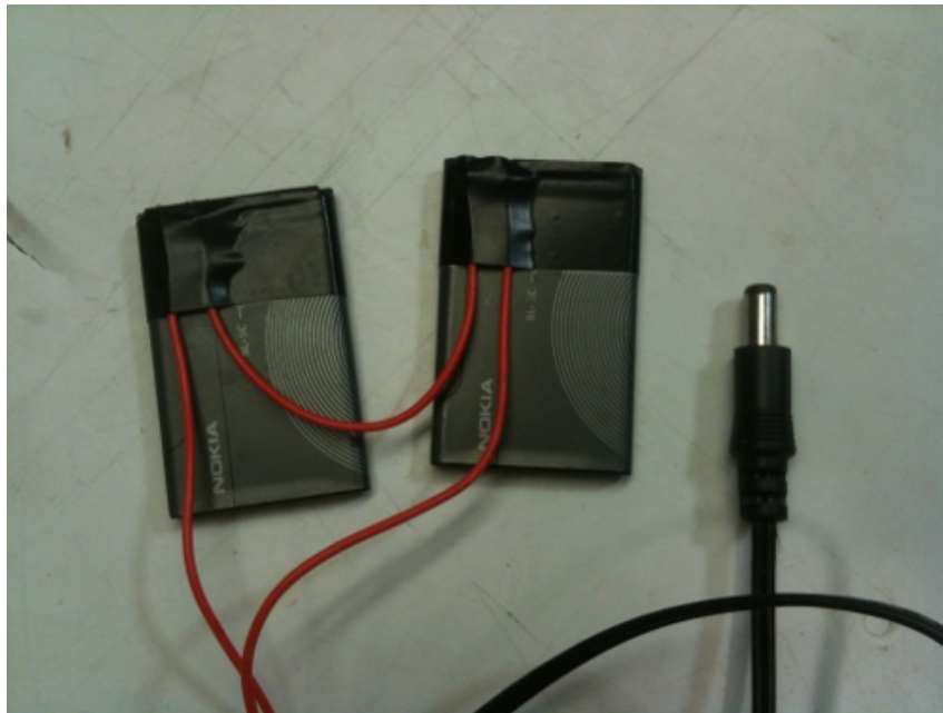
The Completed Battery Pack, with Barrel Plug
